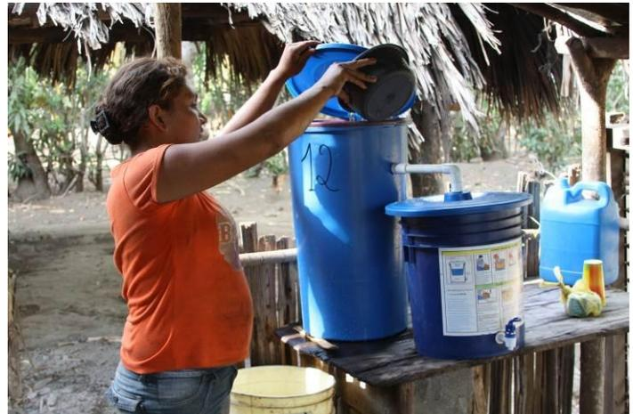
Candida Rosa Moreno from Bella Vista fills a glass of water from her filter. Here the water passes through the Kanchan filter to remove arsenic and is then chlorinated to remove bacteria in the second bucket.
