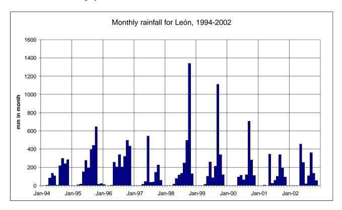
A reasonably conservative estimate of annual rainfall for San Jacinto based on isohyet maps of 1400 mm was used to calculate a typical annual cycle for San Jacinto rescaling the time series data for León. This is shown in the graph below:
