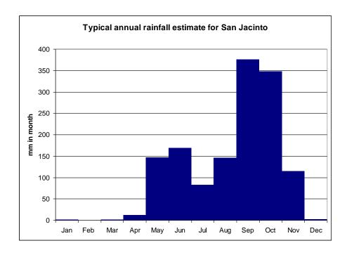
It can be seen from this cycle that there are five months of the year that are effectively completely dry and thus a design criterion for rainwater storage was that the tanks should be large enough to store sufficient water to meet a basic minimum household demand for 150 days. This was calculated for each household using a national standard for rural water supply of 30 litres per person per day.
